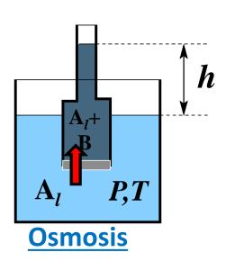
$$\rho gh = \Pi = -\frac{RT}{V_{A,m}^*} \ln a_A$$
